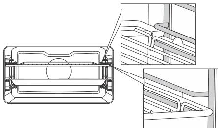
In case of wire guides, always insert the wire rack and the baking tray into the slot between the upper and lower part of each guide level.
