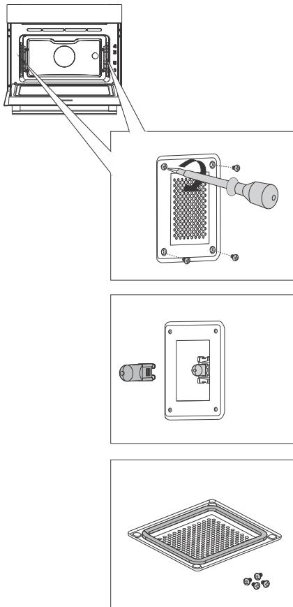
**1** Undo the four screws. Remove the cover and the glass.
