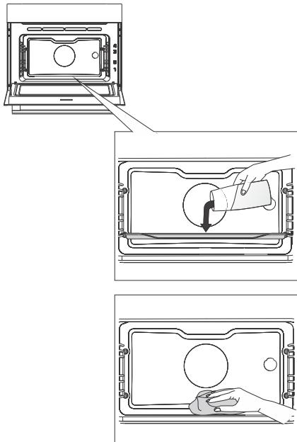
**1** Insert the glass baking dish into the first guide level and pour 1.5 dl of warm water into it.
