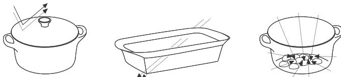
When food is exposed to microwaves, the molecules begin to move rapidly, thereby generating heat. The microwaves penetrate approximately 2.5 cm deep into the food. If the food is thicker, the core of the food will be cooked by conduction, as in conventional cooking.
