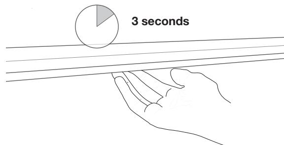
By moving your hand under the sensor, you "scroll" through the available colours. You can scroll forward and backward by moving the hand either from left to right or right to left underneath the sensor.
