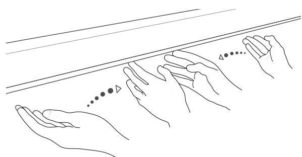
By moving 2 hands away from each other under the sensor strip, you can make the beam wider.
