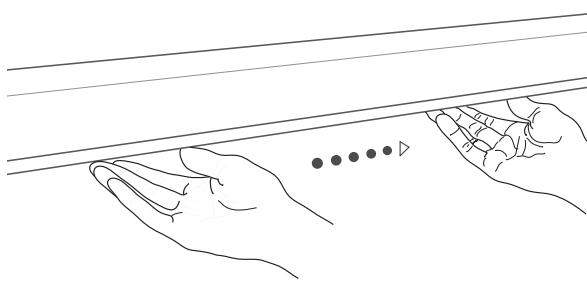
Another way to move the light beam is to hold your hand at the place under the sensor where you want to move the light beam. The light beam will then move towards your hand.
