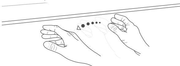
2. A narrower beam is activated by holding your hand under the sensor strip for more than 1 second. The light beam will only be activated at the location of your hand.
