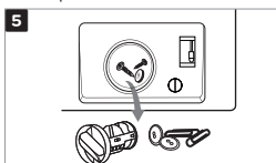
Remove any objects and impurities from the filter housing.
