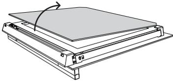
Holding the top of the inner pane, gently pull the pane toward the top of the door until the pane is clear of the notch at the bottom of the door and lift out. Do not angle the pane too much as you may damage the glass.
