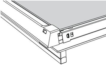
Push the glass retainer tabs in on both sides of the door. Pull the glass retainer up until the tabs relocate in the uppermost hole.
