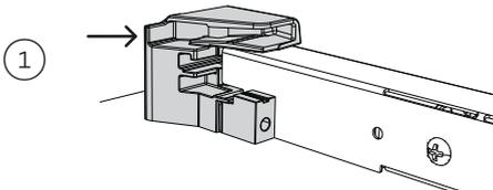
Slide the pane into the notch at the bottom of the door and lower the pane onto the notch at the top of the door.
