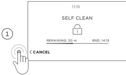
Press the button to the left of the screen at any point during the clean cycle to cancel.
