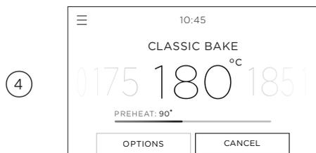
When the oven has reached the set temperature, a tone will sound, the bar will disappear and the dial will turn red.
