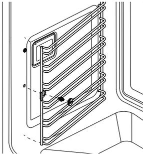
Fit the side rack front tab over the fixing screw.
