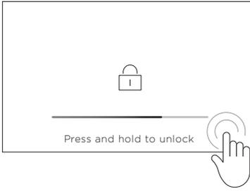
Press and hold anywhere on the screen until the bar fills and the oven unlocks.
