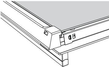
Push the glass retainer tabs in on both sides of the door again. The glass retainer can then be pulled off completely. Gently pull the middle pane toward the top of the door until the pane is clear of the notch at the bottom of the door.
