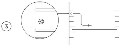
Place food in the oven and plug the sensor into the socket inside the oven, on the left hand side.
