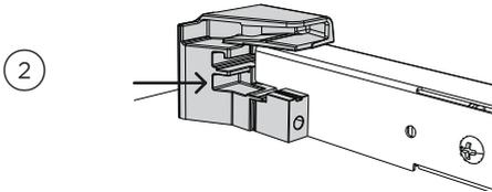
Slot the bottom of the pane into the lower notch at the bottom of the door.
