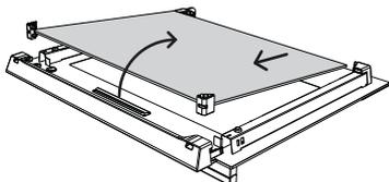
Gently pull the middle pane toward the top of the door until the pane is clear of the notch at the bottom of the door. Lift the pane out. The rubber stoppers at the top of the pane remain attached to the glass pane.
