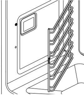
Slide the rear prongs of the side rack back into the holes, ensuring the rack is firmly pushed up against the side wall of the oven.
