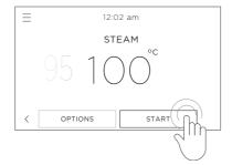
Select the desired steam function and temperature, and press start.
