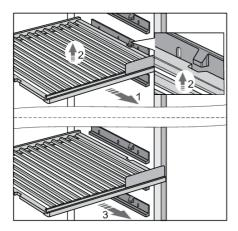
To remove a shelf from the appliance, partly pull it towards you (1) until the two grooves on the shelf and the block on the plastic shelf supports are aligned. Then, lift the shelf (2) and pull it out from the appliance (3). Take care not to damage the door gasket.
