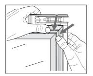
6. Carefully press the gasket back into the groove in the door.
